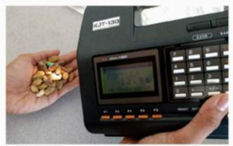
commonly used in grain moisture meters is based on the relationship between a grain's moisture content and its dielectric constant. As its moisture content increases, its dielectric constant increases. Since the rate at which the dielectric constant increases is different for all grain types, a unique calibration is necessary for each grain type.
