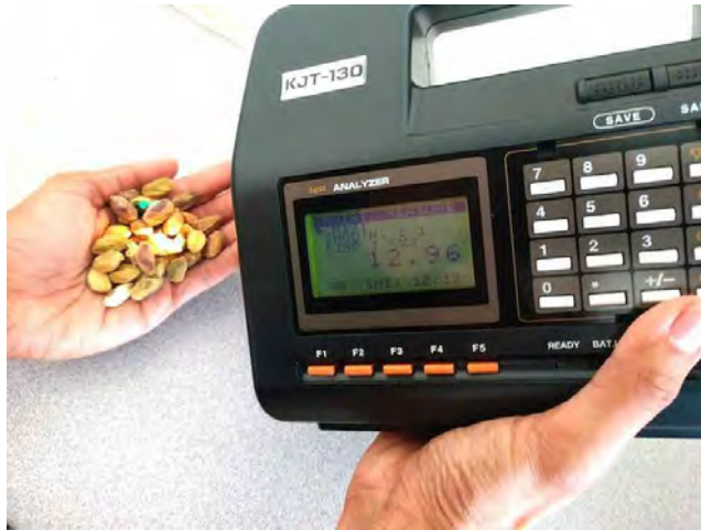
Kett KJT130 portable moisture meter - instant moisture measurement on pistachio nuts
