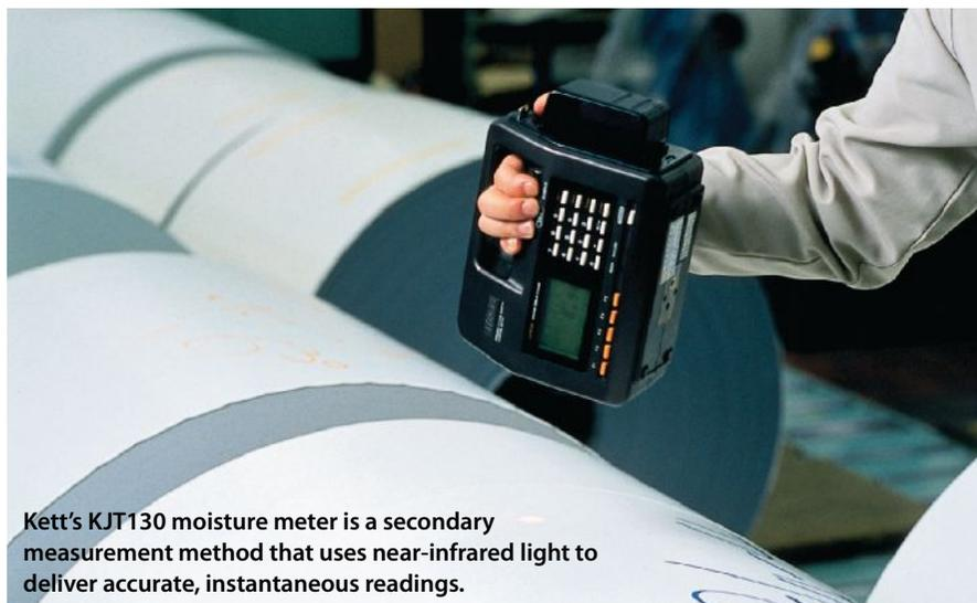
Kett's KJT130 moisture meter is a secondary measurement method that uses near-infrared light to deliver accurate, instantaneous readings.
