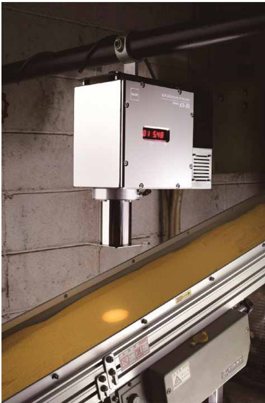
Continuous moisture monitoring by smart technology allows for the tracking of historical performance trends.
