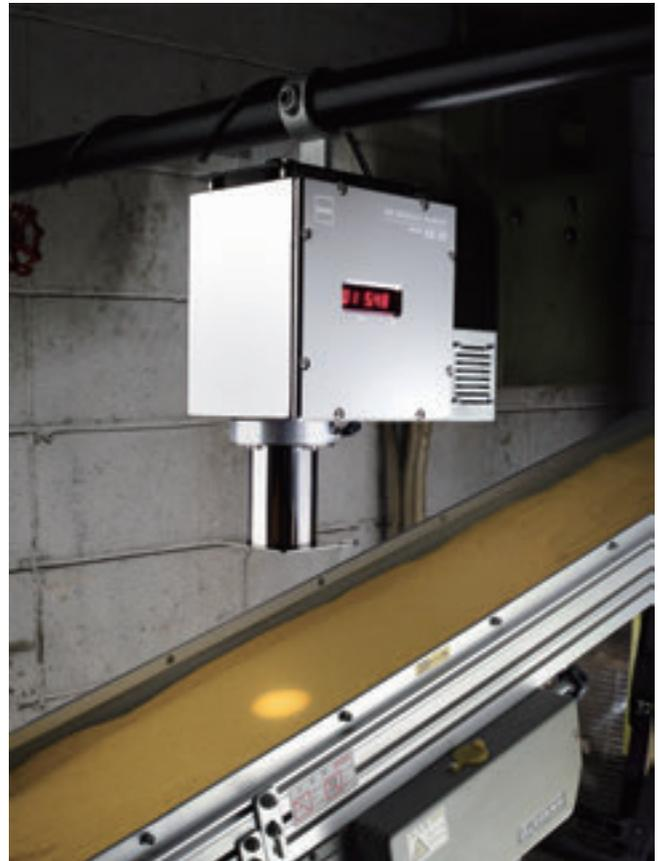
**Continuous moisture monitoring by smart technology allows for the tracking of historical performance trends.**
