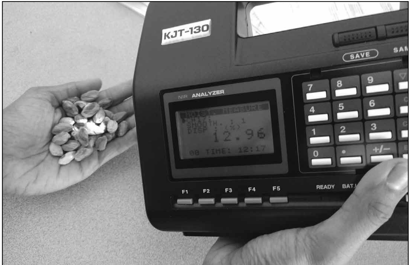
Portable single grain moisture tests can quickly measure the moisture within each grain of rice, barley and wheat, allowing farmers to determine the moisture content of individual seeds within a sample.
