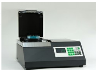
Kett KB270F desktop NIR moisture analyzer.
