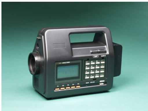
Portable NIR moisture analyzers such as the Kett KJT130 sell for about $16,000.
