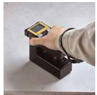
The Kett HI520-2 portable moisture meter for concrete, mortar, and drywall applications
