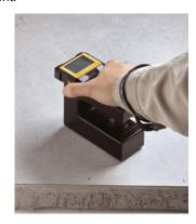
The new tool uses Near-Infrared (NIR) light, a highly accurate, non-contact secondary measurement method that can deliver the moisture readings of solids, slurries, and liquids in seconds without sample preparation in portable handheld models. The meter reflects light off the sample, measures how much light has been absorbed, and automatically converts the result into a moisture content reading.
