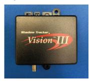
Compared with typical GPS tracking devices that may only update every few minutes, the system provides real-time location updates every 10-seconds, as well as location, speed and idle time alerts if something is amiss. This data is transmitted via satellite and cellular networks to a smartphone or PC on a 24/7 basis. The system has access to nationwide speed limits in its database, which can help deter driver speeding.
