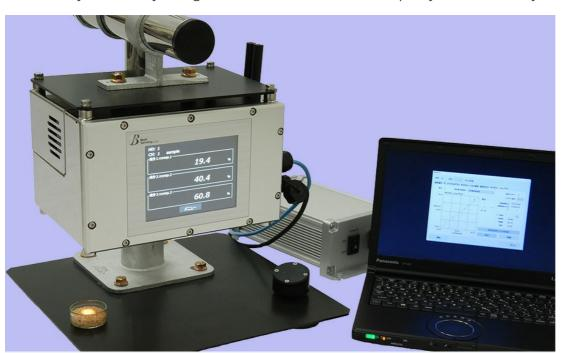
An online near-infrared (NIR) analyzer, such as the Kett BS-R1700, can provide real-time compositional monitoring and analysis of food at a distance of 50 to 100 mm as it passes by on a conveyor, allowing processors to confirm that the foot meets labeling compliance, quality specs and desired consistency. Source: Kett
