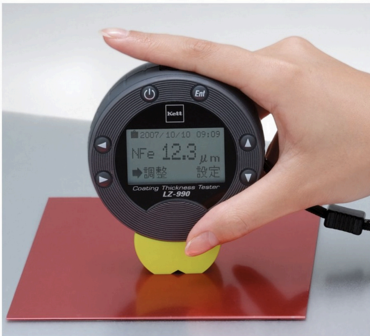
Handheld devices allow personnel to easily and quickly perform lab-quality coating thickness measurements. IMAGES COURTESY OF KETT US
