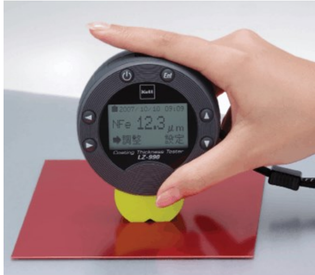
Kett US' LZ-990 coating thickness tester can determine substrates and quickly gage coating thicknesses to 0.1μm, allowing more frequent lineside tests throughout various coating processes.
