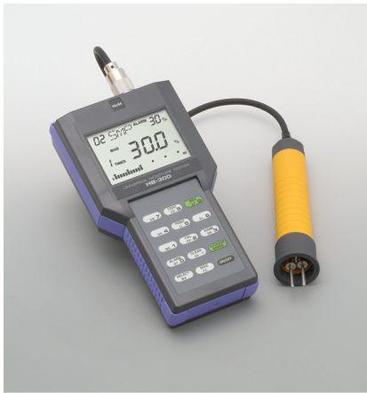
Instant moisture measurement assures speedy results on the jobsite.
