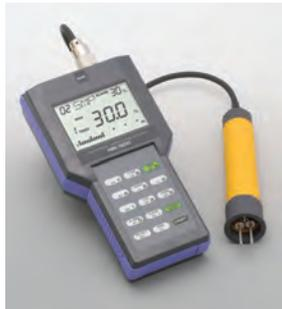
The durable HI520-2 instant moisture meter allows anyone to spot check concrete and mortar at the jobsite to assure that it is properly mixed, set, and dry. It allows non-destructive, non-invasive testing on a digital display with no pin holes or discoloration. This facilitates construction work as soon as feasible, speeds project completion, and improves quality.
