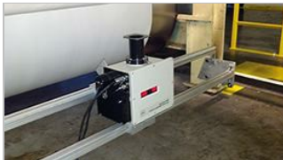
Smart moisture measurement devices enable corrective adjustments to be made
