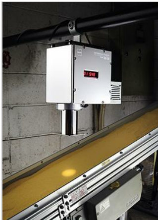
Continuous moisture measurement by smart technology allows for the tracking of historical performance trends
