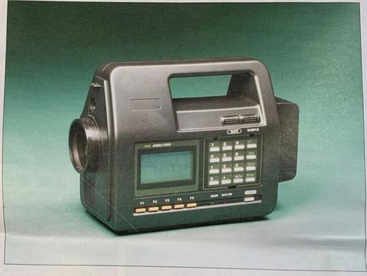
Fortunately, a new category of portable, handheld, instant moisture measurement devices are now available for construction workers that can be used on a wide range of materials with no special training.
