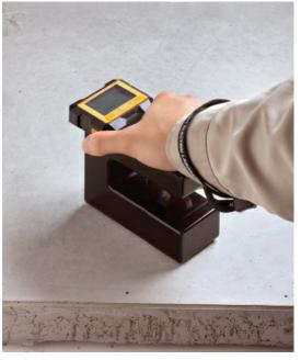
off the sample, measures how much light has been absorbed, and the result is automatically converted into a moisture content reading.
