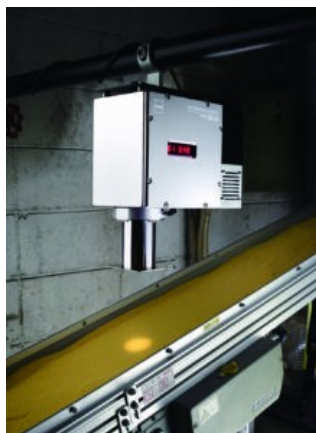
KB30 Online moisture meter – non-contact, non-destructive, instant
