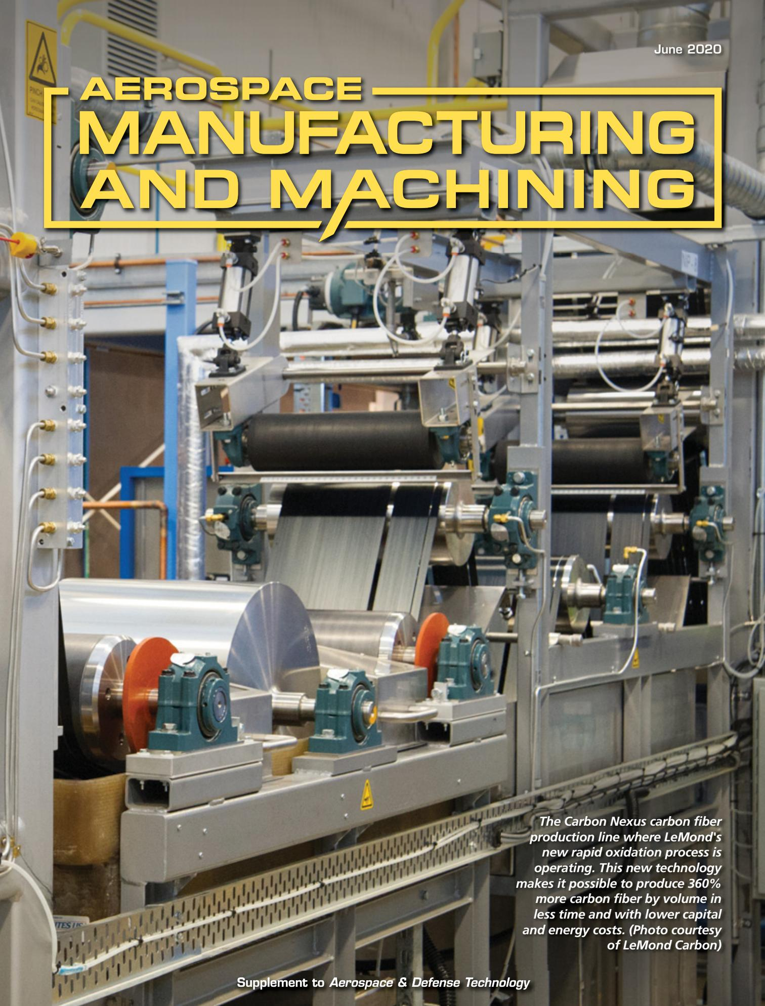
*The Carbon Nexus carbon fiber production line where LeMond's new rapid oxidation process is operating. This new technology makes it possible to produce 360% more carbon fiber by volume in less time and with lower capital and energy costs. (Photo courtesy of LeMond Carbon)*
