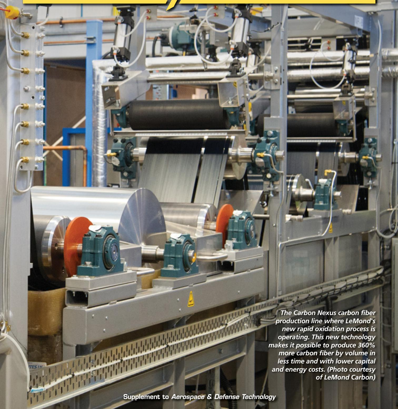
*The Carbon Nexus carbon fiber production line where LeMond's new rapid oxidation process is operating. This new technology makes it possible to produce 360% more carbon fiber by volume in less time and with lower capital and energy costs. (Photo courtesy of LeMond Carbon)*
