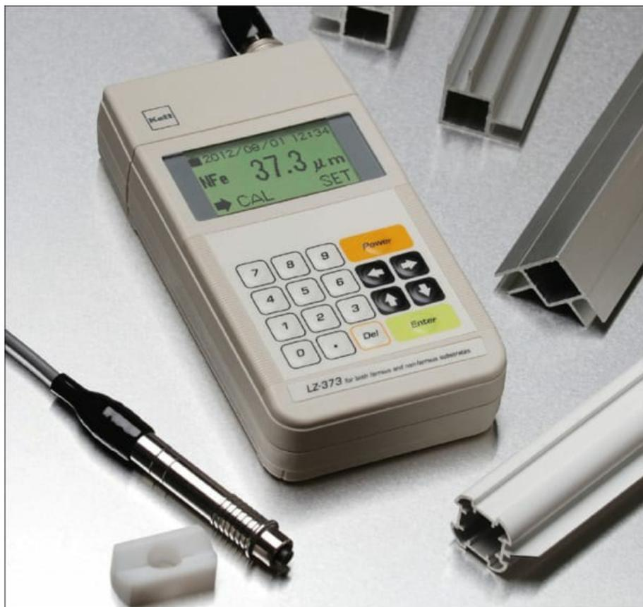
Kett's LZ-373 US aerospace analyzer works on both ferrous and non-ferrous substrates.
