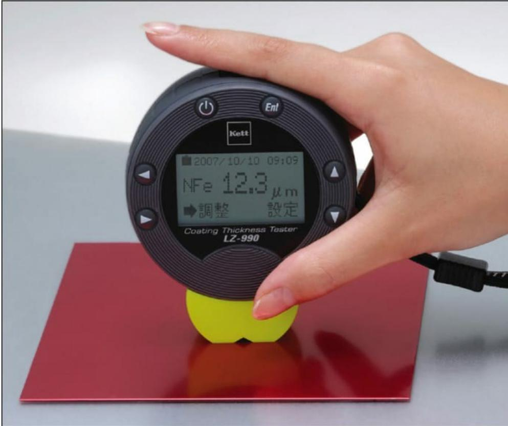
Modern handheld devices like this Kett coatings analyzer are now available to allow personnel to perform lab-quality coating thickness measurements using one hand, even on curved and complex surfaces.
