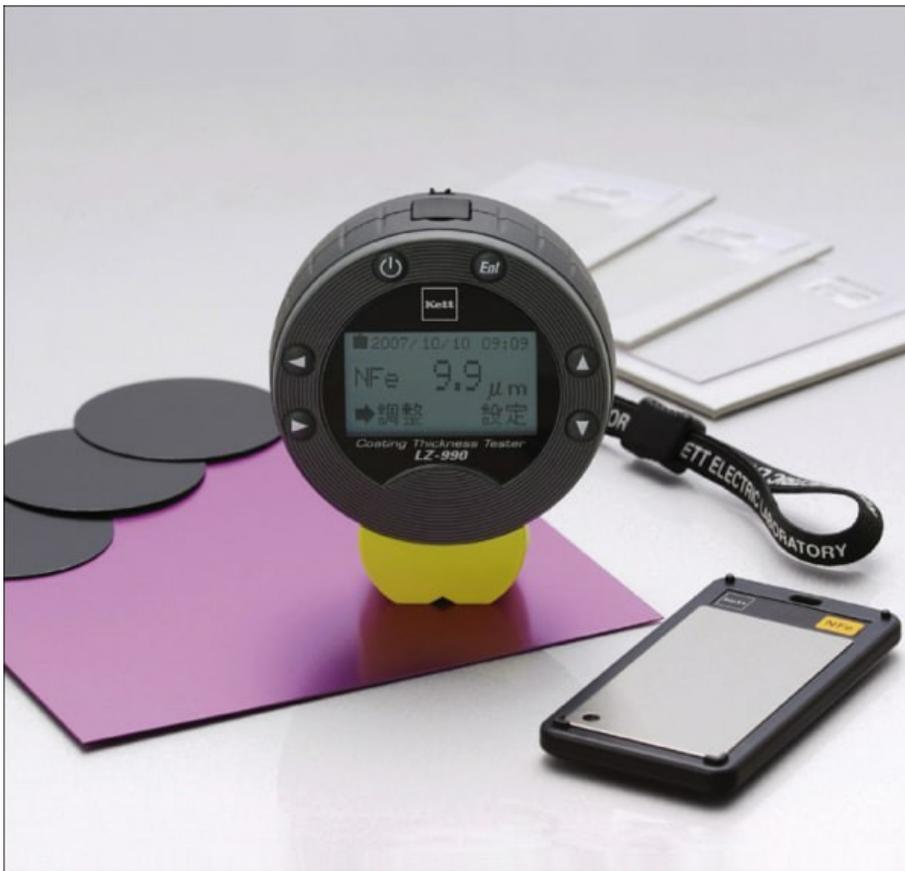
Some instruments offer instant coating thickness measurement of almost any non-magnetic coating on both ferrous (magnetic) and non-ferrous (non-magnetic) substrates.
