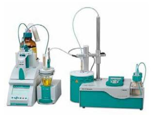
with the initial mass or volume of the sample and the moisture content is calculated. Karl Fischer tests can be very accurate, testing to the Parts Per Million (PPM) level.
